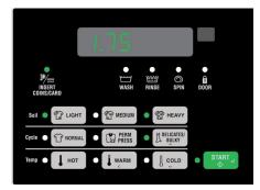
Quantum<sup>®</sup> Control Features: Digital display for vend price and cycle time countdown. Touch pad control with LEDs. Three temperature selections for Hot, Warm or Cold water. Three fabric selections for Normal, Permanent Press or Delicate. Three soil level selections for light, medium, or heavy, offering 27 possible cycles. Push-to-Start activation. LEDs show the cycle and the door lock status. Infrared programming.
