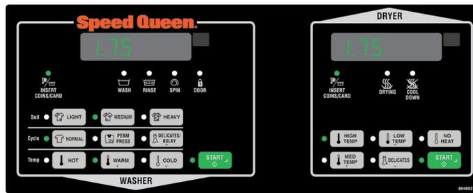
**Quantum® Control Features:** Digital display for vend price and cycle time countdown. Touch pad control with LEDs. Three temperature selections for hot, warm or cold water. Three fabric selections for normal, permanent press or delicate. Three soil level selections for light, medium, or heavy, offering 27 possible cycles. Push-to-Start activation. LEDs show the cycle and the door lock status. Infrared programming. Quantum models available with card or coin start operation.
