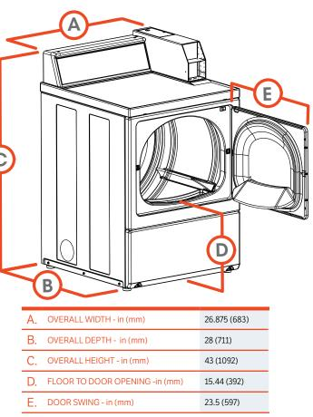
\* Electric dryers come equipped for 240/60/1 operation. They can be field converted to operate on 208/60/1 with optional 61928 conversion kit. Gas dryers can be field converted for operation on LP gas with optional 458P3 conversion kit.
